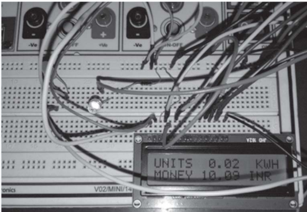
Figure : 01. This model clearly shows the display of money and units consumed when two 100 Watt bulbs have been lit in a parallel connection. The white led in this case shows that the current is within fair limits and the money is also within the limiting value entered by the user.
